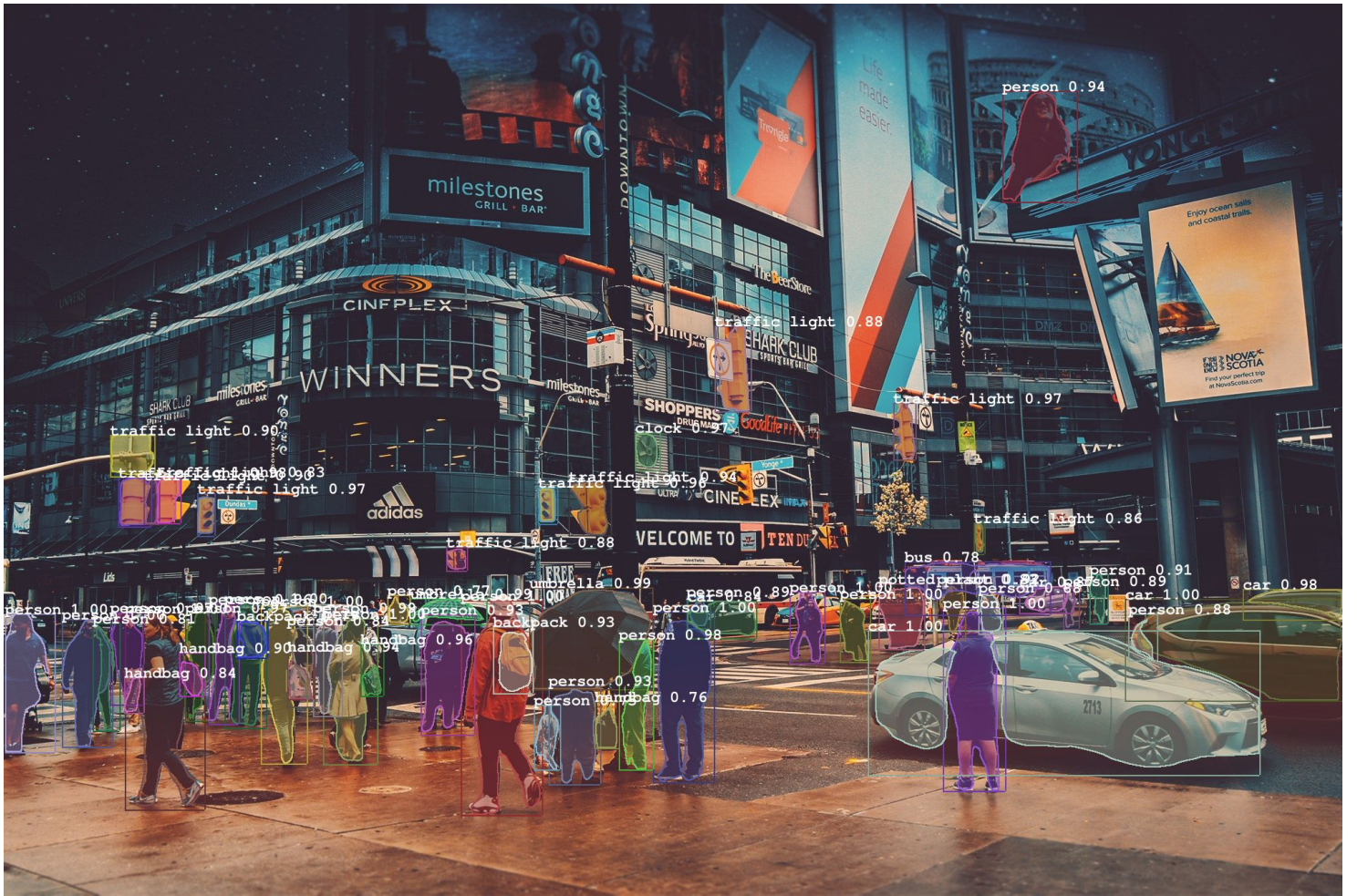
Figure 1: Image processed by the Owl implementation of Mask R-CNN.
